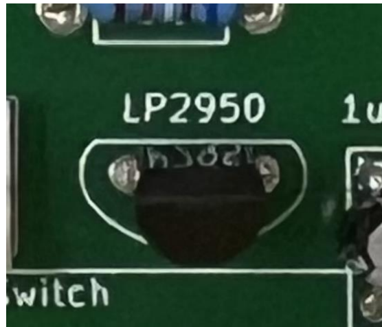
Figure 5.3: LP2950 regulator on the PCB.
