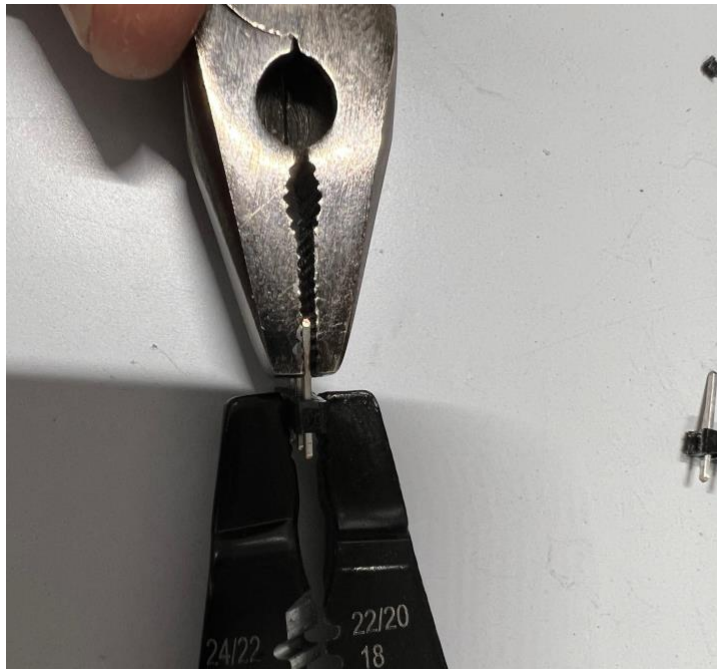
Figure 2.1: Pulling out the metal pins from male breakaway pins.
