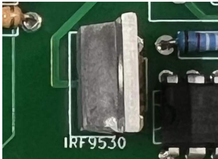
Figure 5.4: IRF9530 transistor on the PCB.
