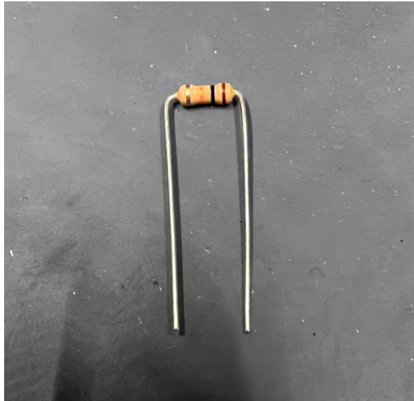
Figure 3.1: Bending resistor leads to insert into the PCB.
