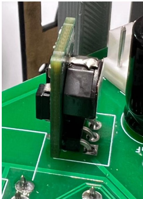
Figure 5.2: OKI-78SR regulator on the PCB.
