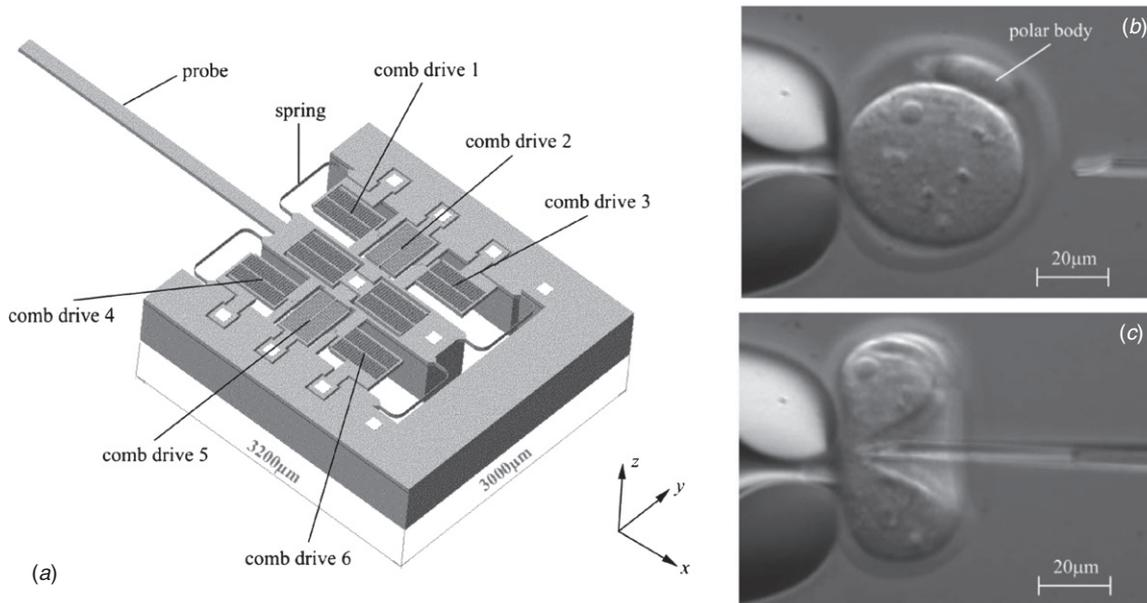
**Figure 5.** (a) Schematic of a dual-axis feedback controlled electrostatic actuator. The comb-drive actuators, which remain in air, are used for actuation and capacitive sensors are used for force measurement. (b) Image of an undeformed mouse embryo zone pellucida. (c) A deformed mouse embryo zone pellucida. The applied force is  $12.7 \mu\text{N}$ , and the indenter displacement is  $52.3 \mu\text{m}$ . Images reprinted from [44]. Copyright © 2003 IEEE, with permission.
