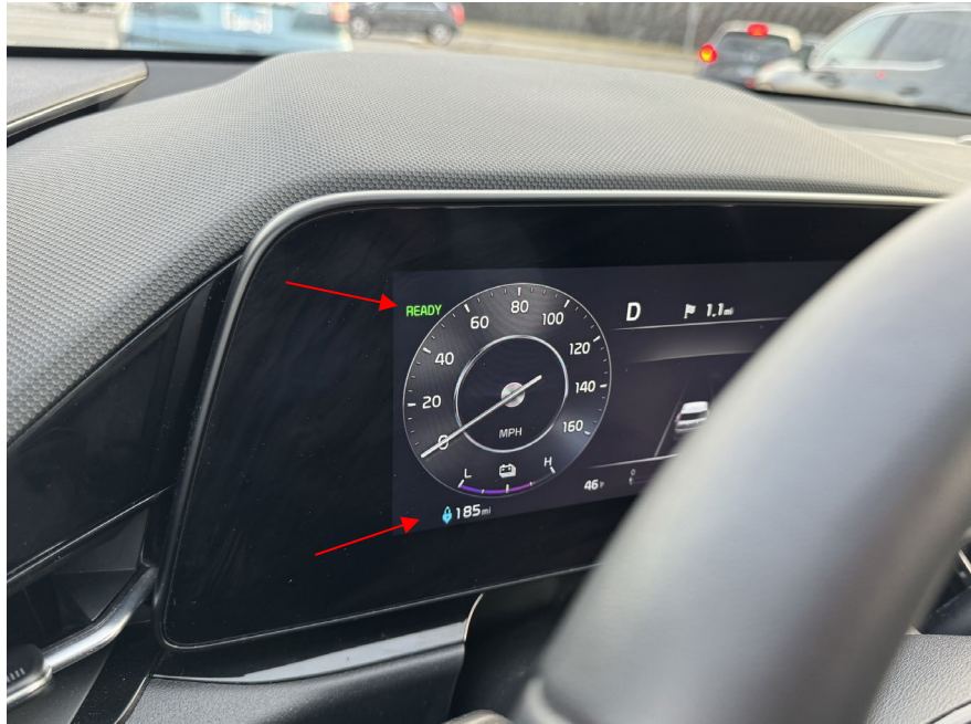
Figure 11 Instrument panel of a Kia Niro, as viewed from the driver's side doorway. Note the green "READY" indicating that the HV battery can supply power to the inverter/wheels, air conditioning, or other HV consumers.
