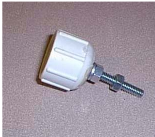
Figure 2.2 a) Fixture that grips the fiber, pinned to the load cell. b) Fixture that holds the mold at the bottom, anchored to the testing machine.
