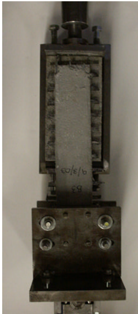
Figure 4.2b Bond test setup with the sample placed in the fixture
