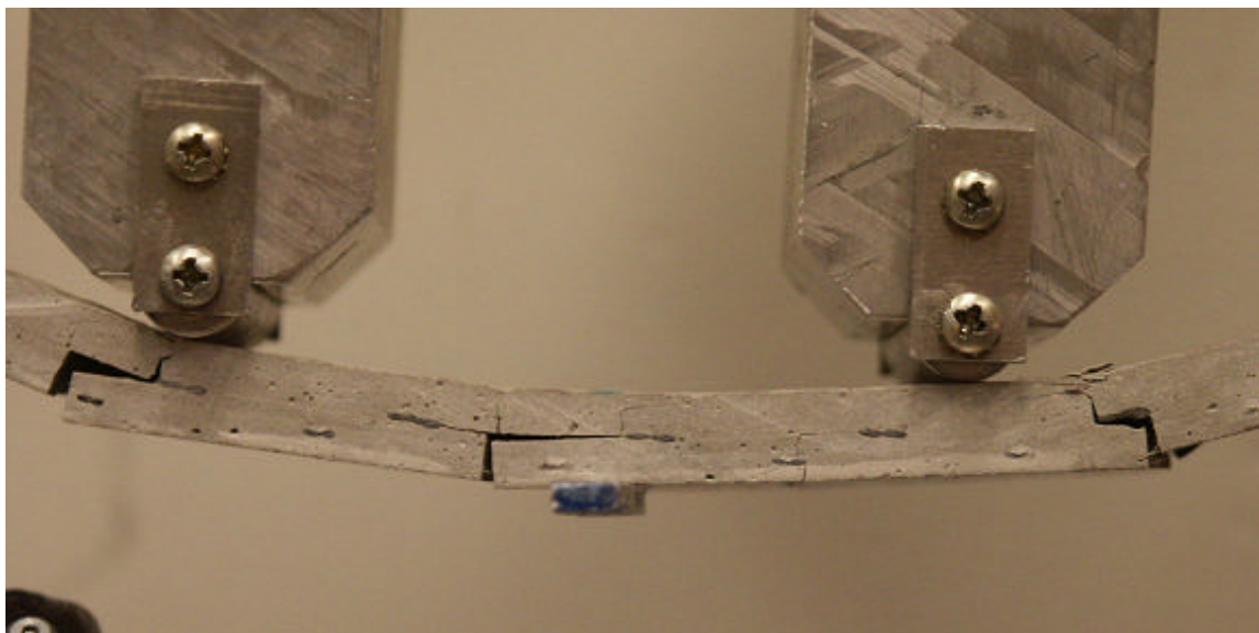
Figure A -29 Figure showing crack formation during flexure test and shows how the crack propagates along the fabric rather than going through and through the matrix and crack it
