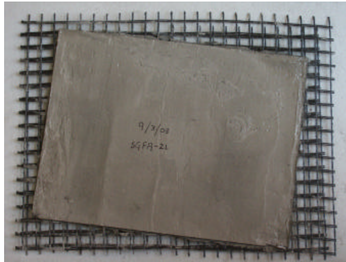
Figure 2.6a) Base plate with 4 strips forming the border, b) Initial layer of an off-axis sample, c) cast of a sample with 2 layers of fabric and a 2 inch offset orientation, d) The de-molded sample.
