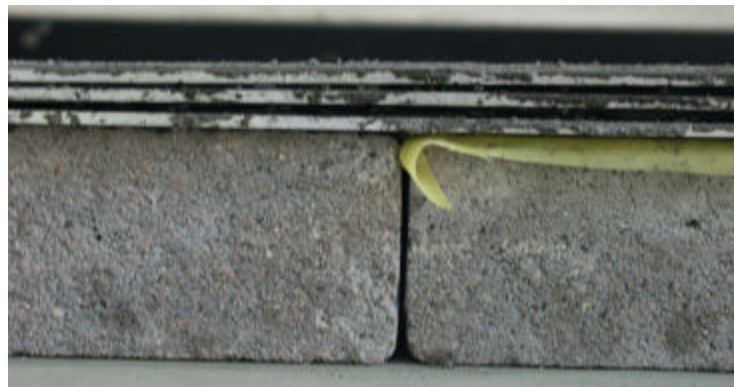
Figure 4.1a Casting of bond sample on 2 masonry blocks. The block covered with yellow sheet (bond breaker) will be removed after initial curing of 24 hours.
