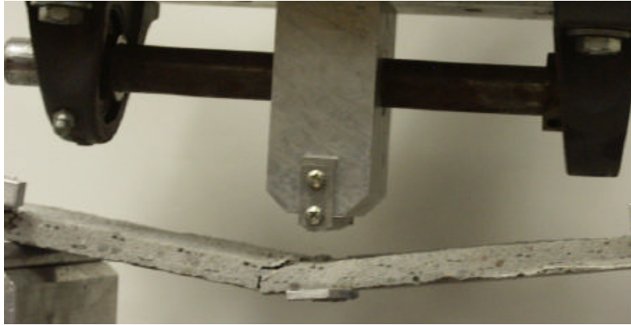
Figure 3.2c Test completed, Load cell is going back
