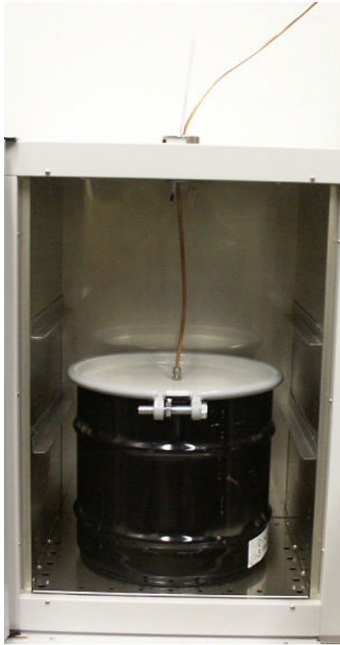
Figure 5.1 Ageing Setup (from Inside the oven) showing the container as well thermometer and copper tube
