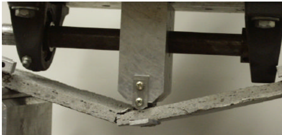
Figure 3.2b Test very near to completion, LVDT has been removed
