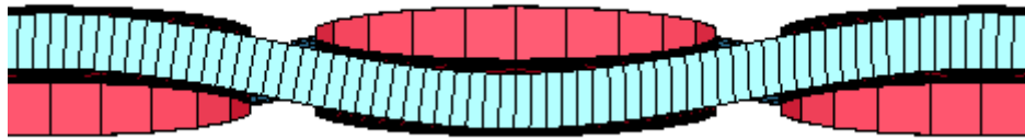
Figure 4.19. (a) Fill yarn longitudinal; cross-section at the start of simulation
