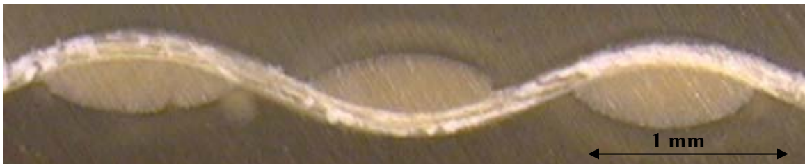
Figure 4.20. (d) Fill yarn longitudinal cross-section under 2.0% Strain level
