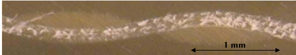
Figure 3.10 (a). Warp yarn longitudinal cross-section – undeformed geometry
