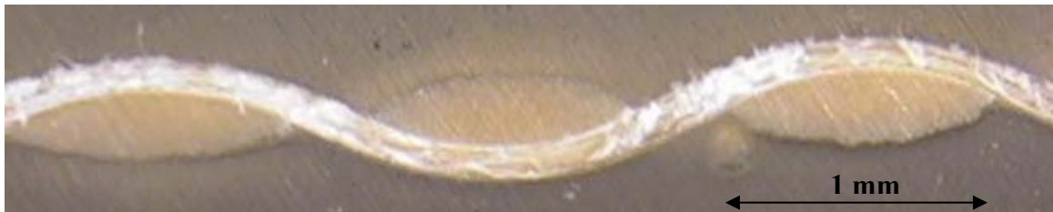
Figure 4.20. (c) Fill yarn longitudinal cross-section under 1.5% Strain level
