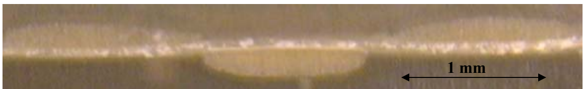
Figure 4.18 (b). Warp yarn longitudinal cross-section under 1.0% Strain level
