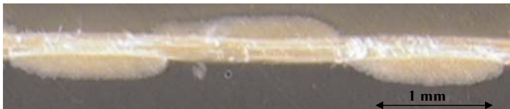
Figure 3.10 (c). Warp yarn longitudinal cross-section under 1.5% Strain level
