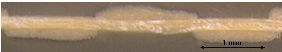
Figure 4.18 (d). Warp yarn longitudinal cross-section under 2.0% Strain level
