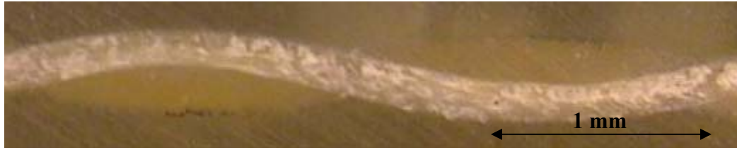
Figure 3.9 (a). Fill yarn longitudinal cross-section – undeformed geometry
