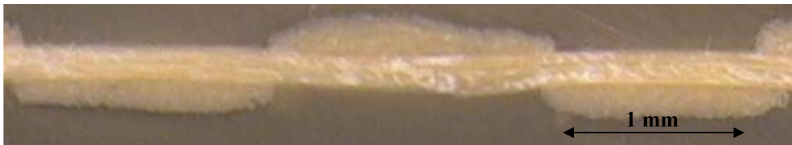
Figure 3.10 (d). Warp yarn longitudinal cross-section under 2.0% Strain level
