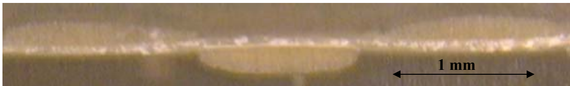
Figure 3.10 (b). Warp yarn longitudinal cross-section under 1.0% Strain level
