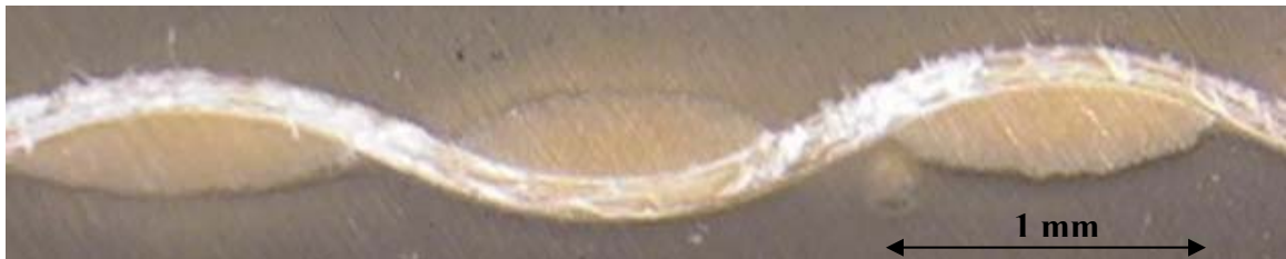
Figure 3.9 (c). Fill yarn longitudinal cross-section under 1.5% Strain level
