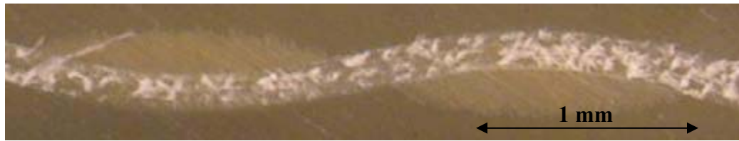
Figure 4.18 (a). Warp yarn longitudinal cross-section – undeformed geometry
