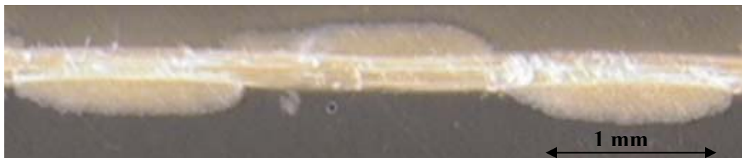
Figure 4.18 (c). Warp yarn longitudinal cross-section under 1.5% Strain level
