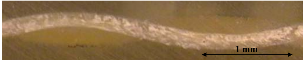
Figure 4.20. (a) Fill yarn longitudinal cross-section – undeformed geometry
