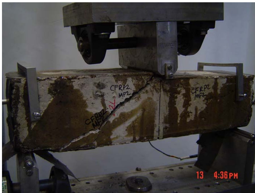
Figure 5.2.3.3. Failed CFRP 2 layers retrofitted sample
