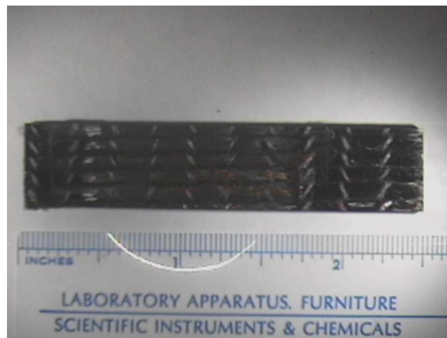
Figure 2.4.2.1. Typical Uniaxial Compression CF sample (2 cloth layers)
