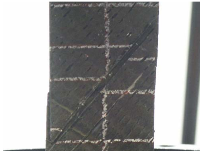
Figure 2.4.3.8. CFC failure pattern under +/-45 shear test
