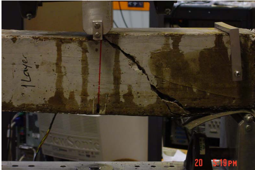
Figure 5.2.3.2. Failed CFRP 1 layer retrofitted sample
