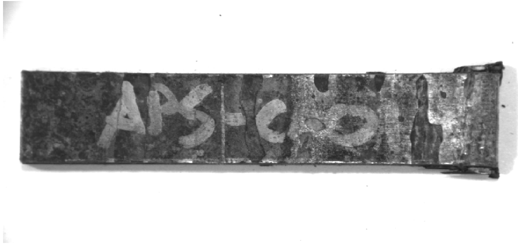
Figure 2.4.2.9. Crushing of the lower part under uniaxial compression
