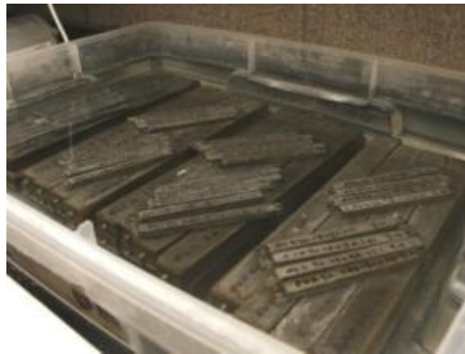
Figure.4.4.1 Sample A and Sample B Specimens in Sodium Sulfate solution
