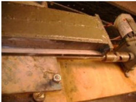
Figure C: vibrating the cast molds
