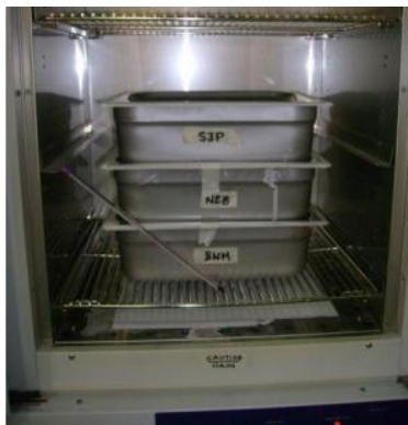
Figure.4.4.2 Specimens in Sodium hydroxide solution in Owen at 80^{\circ}\text{C}
