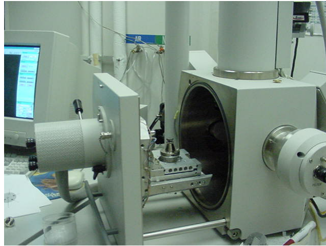
Figure.2.3.2 SEM Chamber where the samples are loaded ( http://wikipedia.org )
