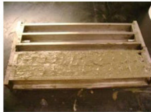
Figure B: casting the bars with mortar
