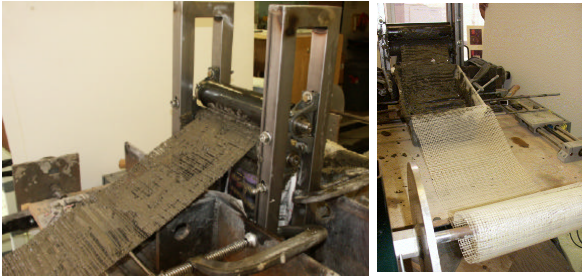
Fig. 2.3. Manufacturing of fabric cement composites with the pultrusion process
