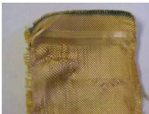
Figure 2.40: Failure at the edge
