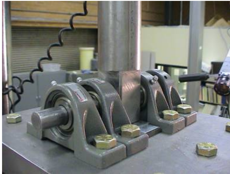
Figure 3.6: Top plate with bearings orthogonal to nose bearings (Fixed end condition at top)
