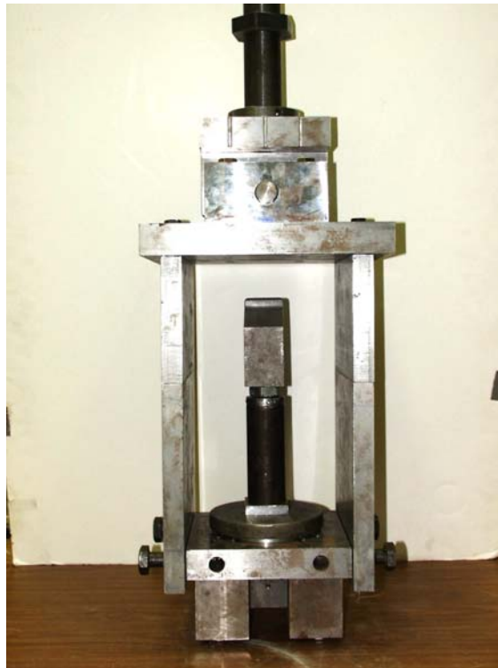
Figure 3.7: Blunt nose housing design (fixed-fixed conditions)
