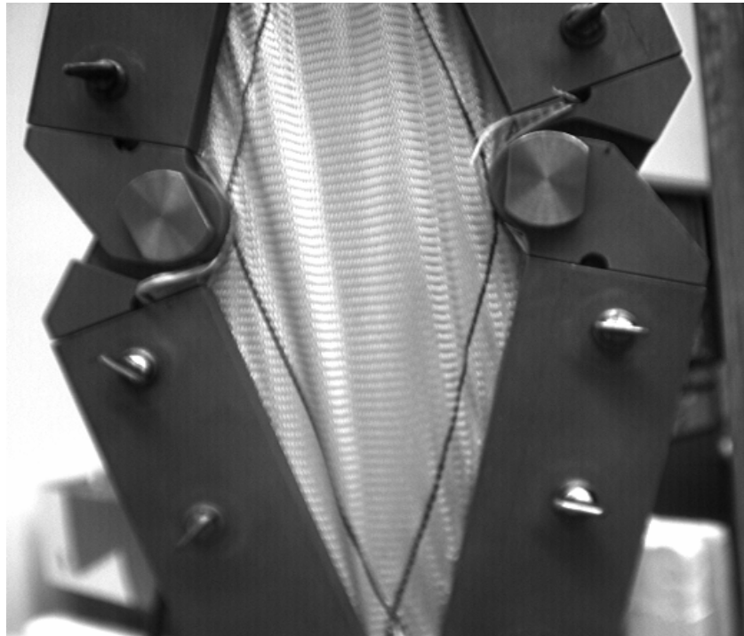
Figure 5.31: Kevlar Test Fabric for Picture Frame Tests in Final Stage of Loading
