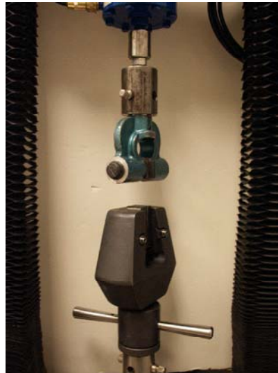
Fig. 3.7. Setup for pullout test
