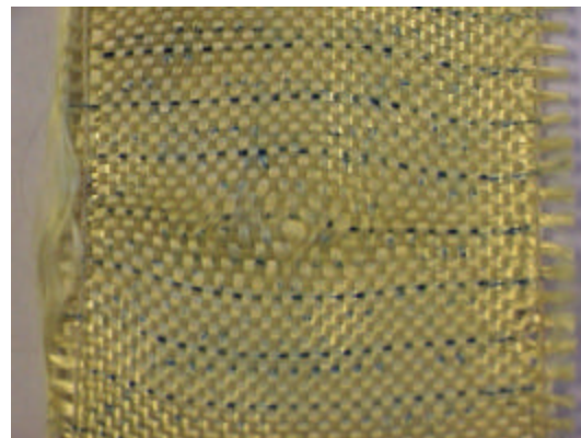
Figure 2.38: Failure at center
