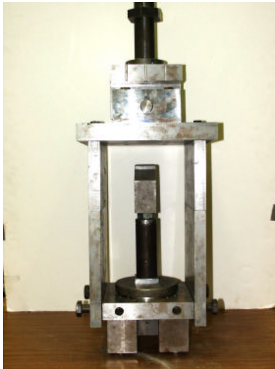
Figure 3.7: Blunt nose housing design (fixed-fixed conditions)
