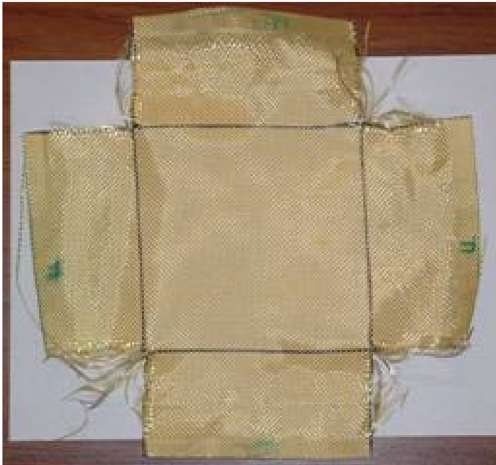
Figure 5.26: Kevlar Test Fabric for Picture Frame Tests
