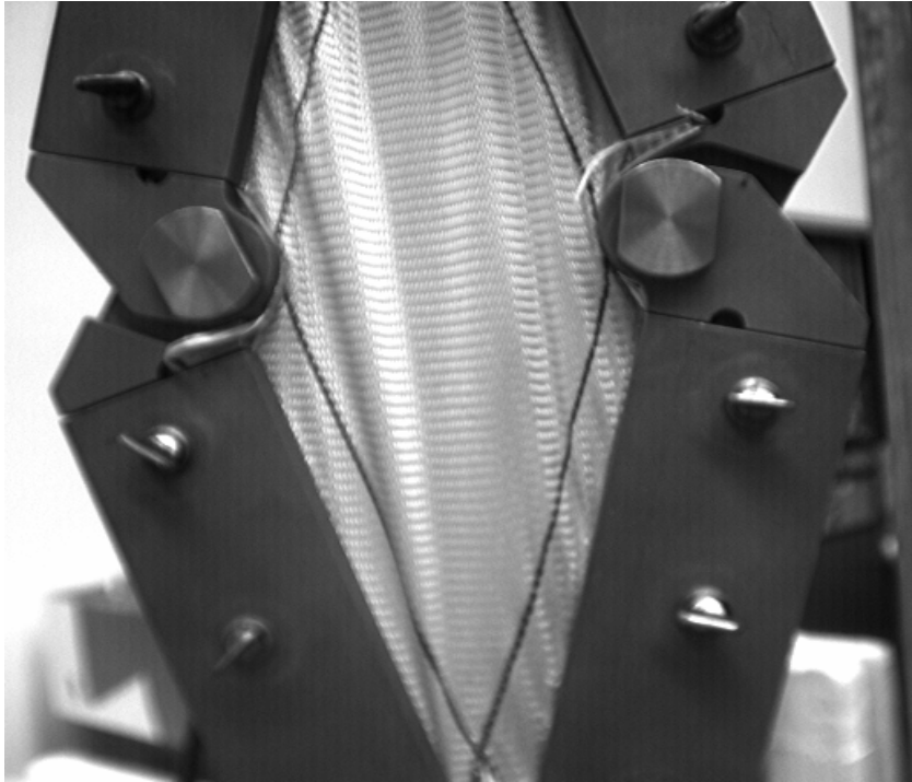
Figure 5.30: Kevlar Test Fabric for Picture Frame Tests in Final Stage of Loading
