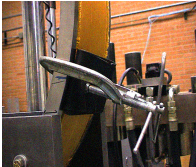
Figure 3.8: Attachment of C-clamps to the specimen
