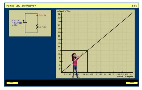
Fig. 2. Sample screen shot of multi-representation display screen with Ohm's Law equation calculations, a circuit diagram, and a Cartesian graph of voltage as a function of current used in the simulation session.
