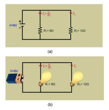
Fig. 1. Sample circuit diagrams from both the no labels (N) conditions: Only the variables denoting the circuit quantities are included in the diagram. There are no text labels that explain the meanings of the symbols for the circuit components in the abstract representation or the illustrations of the circuit components in the contextualized representation. (a) Abstract representation (A). (b) Contextualized representation (C).
