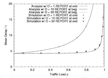
Fig. 5. Mean delay versus mean aggregate throughput for different numbers of ONUs O and reporting at the *end* of an upstream transmission.
