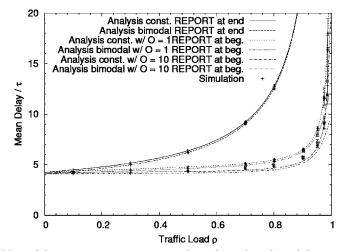
Fig. 7. Mean delay versus mean aggregate throughput for a bimodal versus the constant packet size distribution.
