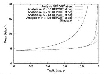
Fig. 3. Mean delay versus mean aggregate throughput for a single ONU. The analytical delay results for reporting at the *beginning* of an upstream transmission are plotted for different maximally considered cycle lengths K.
