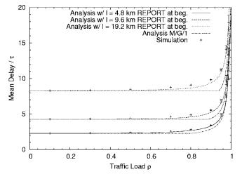
Fig. 6. Mean delay versus mean aggregate throughput for different fiber lengths  $\ell$  and reporting at the *beginning* of an upstream transmission.
