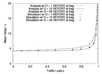
Fig. 4. Mean delay versus mean aggregate throughput for different numbers of ONUs *O* and reporting at the *beginning* of an upstream transmission.
