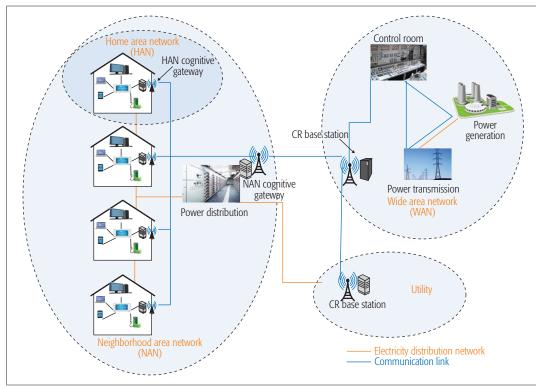
CRNs have to search opportunistically for spectrum access in order to successfully transfer information. In particular, the physical layer should provide statistical information related to channel conditions to the upper layers.
