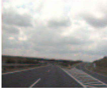
Figure 10: Small quantization parameter ( Q = 16 , PSNR = 44.9579 dB, frame size= 4640 byte).
