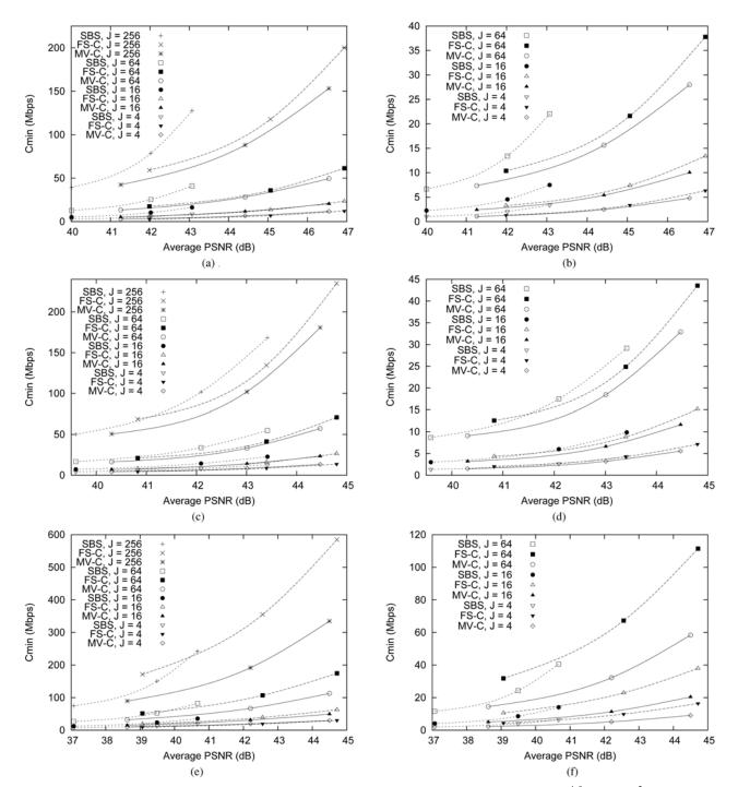
Fig. 3. Required minimum link transmission bit rate  $C_{\min}$  to transmit J streams with an information loss probability  $P_{loss}^{info} \le \epsilon = 10^{-5}$ . (a) Monsters Versus Aliens, frame-by-frame. (b) Monsters Versus Aliens, GoP smoothing. (c) Alice in Wonderland, frame-by-frame. (d) Alice in Wonderland, GoP smoothing. (e) IMAX Space Station, frame-by-frame. (f) IMAX Space Station, GoP smoothing.
