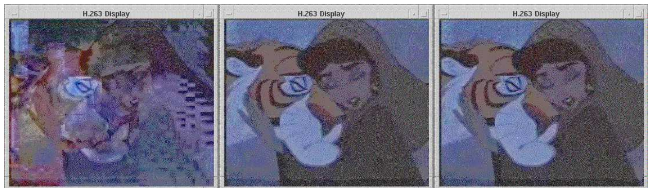
Figure 11: Comparison I of video sequence Aladdin (©DISNEY) after sequential (left), SMPT (middle), and error-free (right) transmission.
