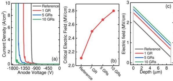
**Fig. 3.** (a) Reverse breakdown measurements for the reference sample and samples with different GRs by Tektronix 370A curve tracer. (b) The critical electric field for the four samples. (c) The calculated electric field profiles of the four samples along the vertical direction of the p-n diodes.
