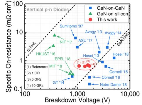
**Fig. 4.**  $R_{on}$  versus  $BV$  of vertical GaN p-n diodes on silicon and GaN substrates [7]–[20]. As-reported values are used for all the references except that  $R_{on}$  in Ref. [18] and [19] were recalculated using the anode for a direct comparison based on [41] and [42]. The circled region shows the devices in this work.
