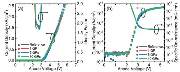
**Fig. 2.** (a) Current density and ideality factor as a function of anode voltage for the reference sample and GaN p-n diodes with different GRs in a linear scale. (b) Current density and  $R_{on}$  versus anode voltage for the reference sample and GaN p-n diodes with different GRs in a semi-log scale.
