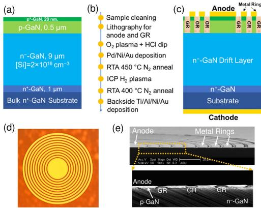
**Fig. 1.** (a) Schematic view of the cross-section of the epilayers. (b) Fabrication process for the devices with GRs. (c) Cross-sectional schematics of the devices with GRs. (d) Optical microscopy image (top-view) of the p-n diodes with 10 GRs. (e) SEM images of the cross-section of the devices with GRs.
