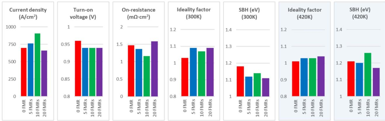
**FIGURE 5.** Device forward characteristics for the SBDs with 0/5/10/20 FMRs. Despite the trivial differences caused by non-uniformity of the material quality and the process fabrication skills, their forward performance is similar enough for a fair comparison of the reverse breakdown measurement.
